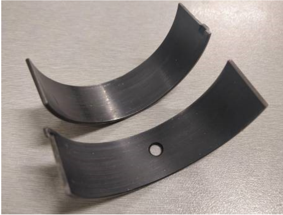
Fig.11 Top Fuel Coated (TFC) Bearings after Top Fuel Race
