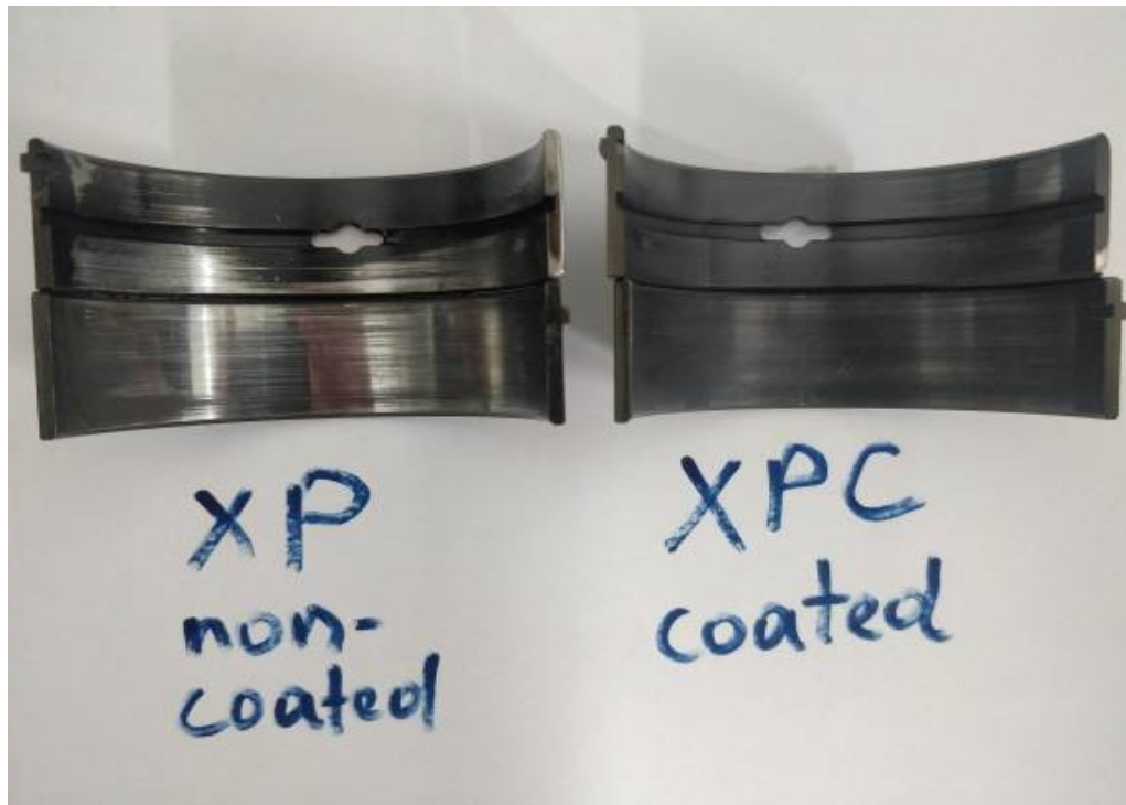
Fig.6 pMax Black™ (left) vs. pMax Kote™ (right) Main Bearings
