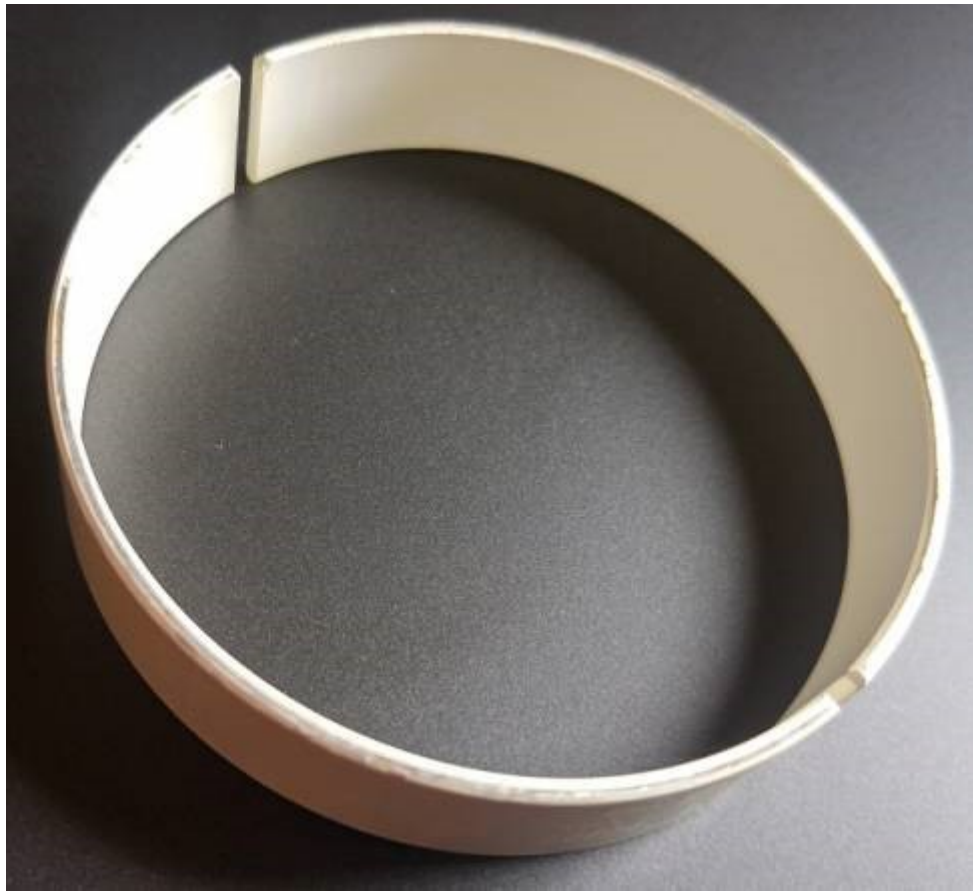
Fig.8 Silver Bearings before Polymer Coating Deposition
